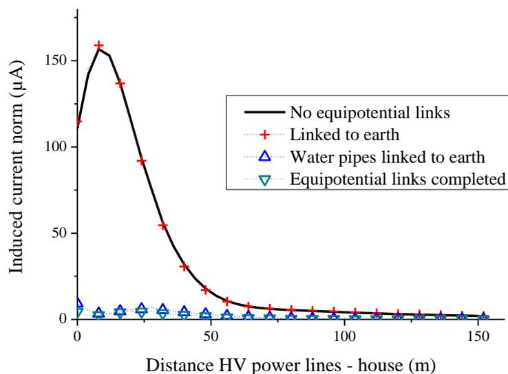
**Figure 29: Critical case of contact current level in a bathtub (Ground loop).**
