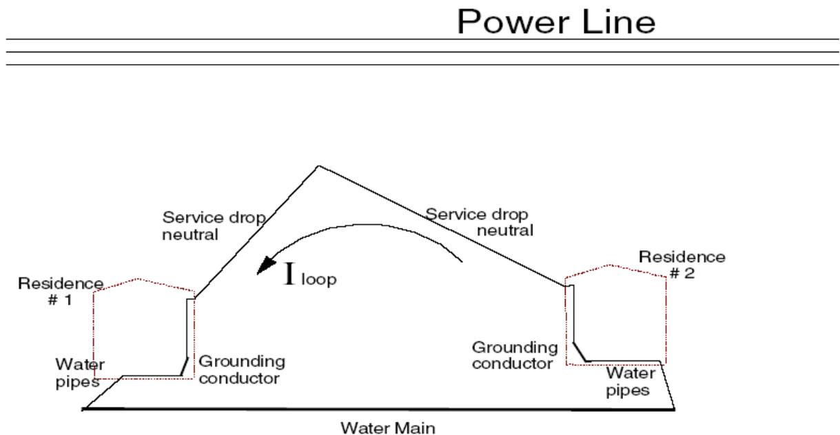
**Figure 20: Current induced in a conductive loop by a power line.**
