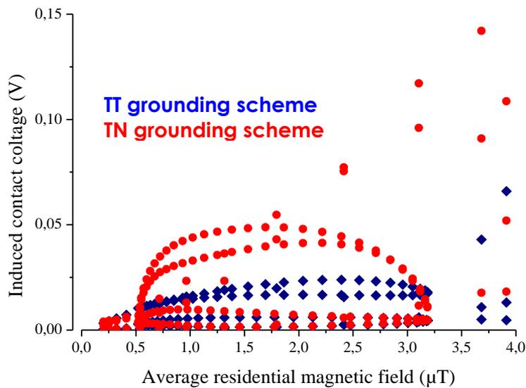
**Figure 28: Contact voltage comparison in a bathtub in TN & TT grounding scheme in groups of houses with ground stakes.**
