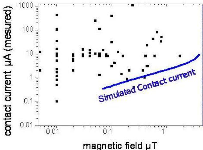
**Figure 38 : Simulated contact current for magnetic field compared to measured cases in Belgium**
