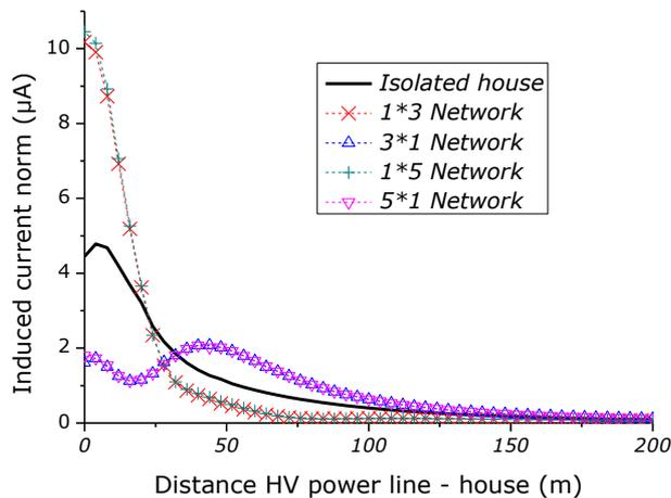
**Figure 11 : Induced current in connection 1 for different networks of houses.**
