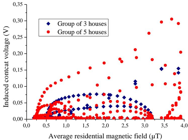
**Figure 31: Induced contact voltage level in function of the size of the group of houses with a TN grounding scheme.**
