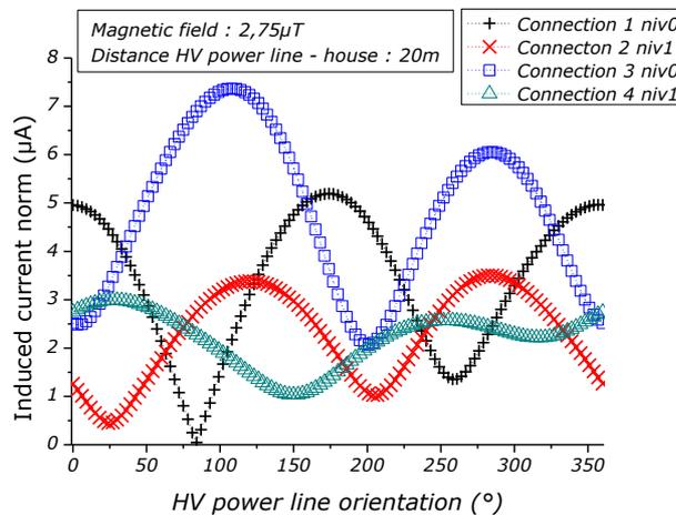
**Figure 5 : Induced current level in a single house as a function of the HV power line orientation.**
