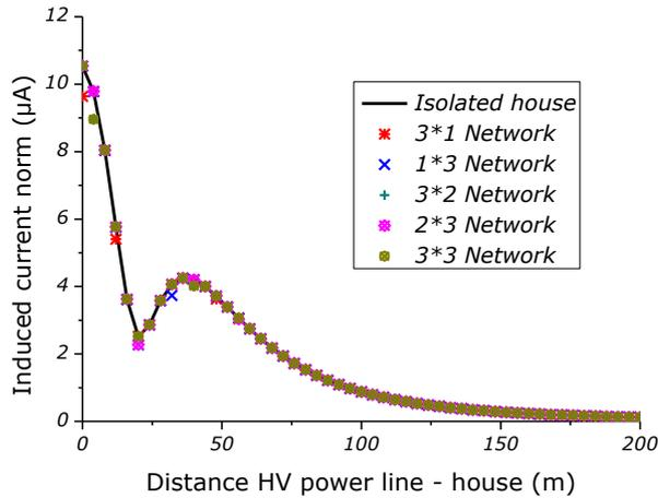
**Figure 10 : Comparison of induced current level in houses in different networks.**
