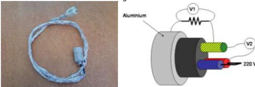
**Figure 42 : three wires low voltage cable (Two wires (phase -bleu;neutral - red) and earth) as used in many houses. With applied 230 V and evaluation of leakage current**
