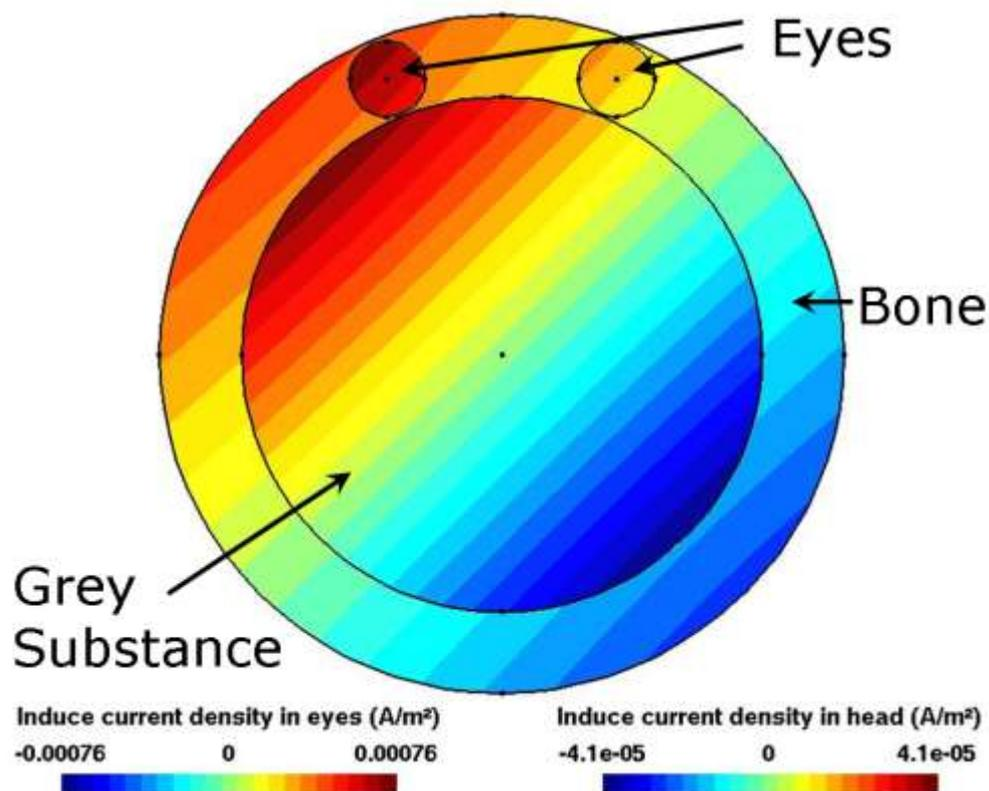
**Figure 2 : Induced current density with maximum induction ( $\sim 20\mu\text{T}$ ).**
