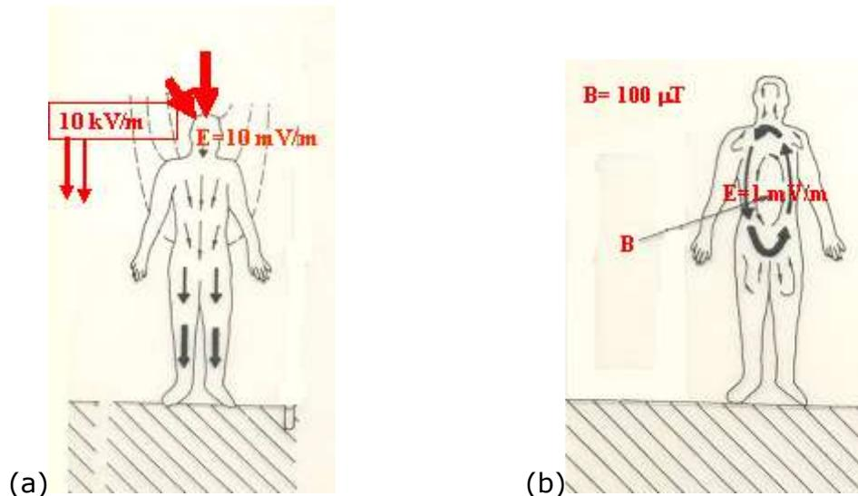
**Figure 48: External E-field (a) and B field (b) effect on human being and resultant internal current and E-field due to current densities appearing into the body. The large arrows on the head (a) indicate a significant increase of the external E-field (compared to ambient field) due to peak effect ( a factor 10)**
