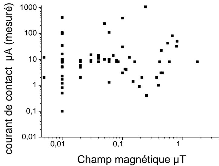
**Figure 37 : Contact current versus magnetic field**
