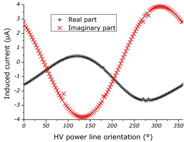
**Figure 6: Real and imaginary part of the induced current in connection 1 in Figure 5.**
