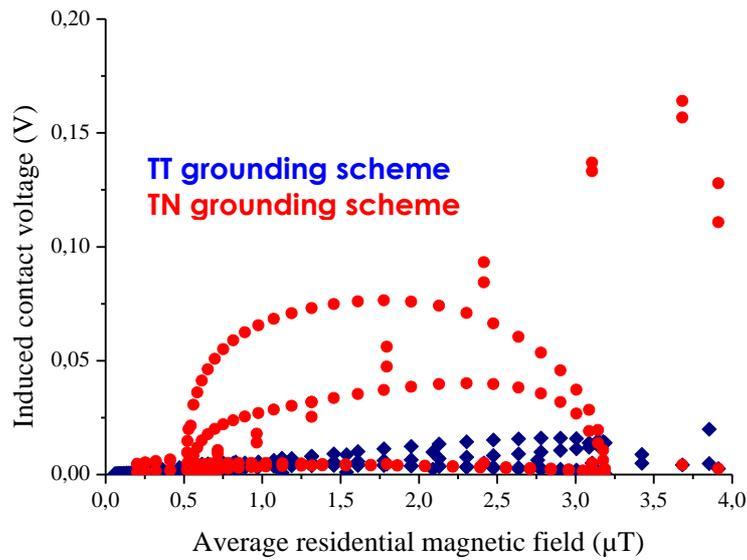
**Figure 26: Contact voltage comparison in a bathtub in TN & TT grounding scheme in groups of houses with ground loop.**
