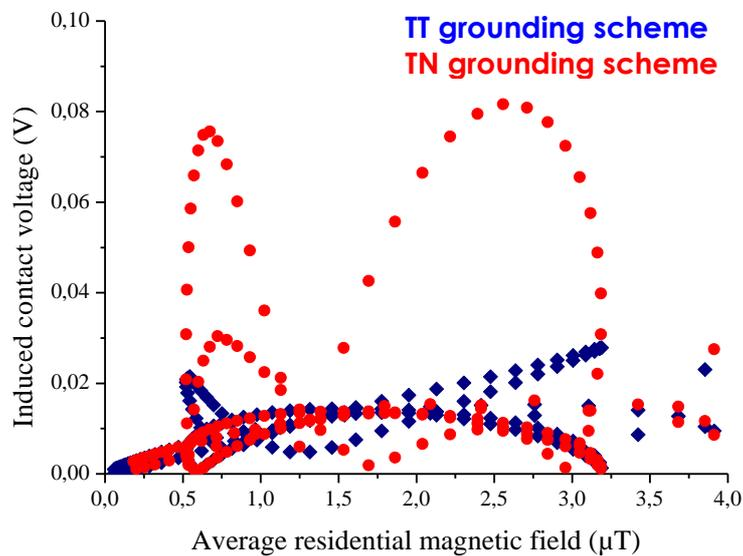
**Figure 25: Contact voltage comparison at a washing machine in TN & TT grounding scheme in groups of houses with ground loop.**
