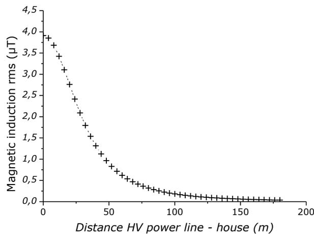
**Figure 3 : Magnetic induction of the HV power line in function of the distance.**
