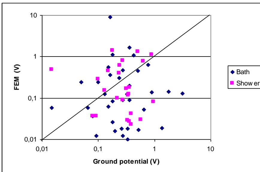
**Figure 39: Belgium campaign. Comparison between the ground potential and the Thevenin equivalent voltages as deduced from measurements.**
