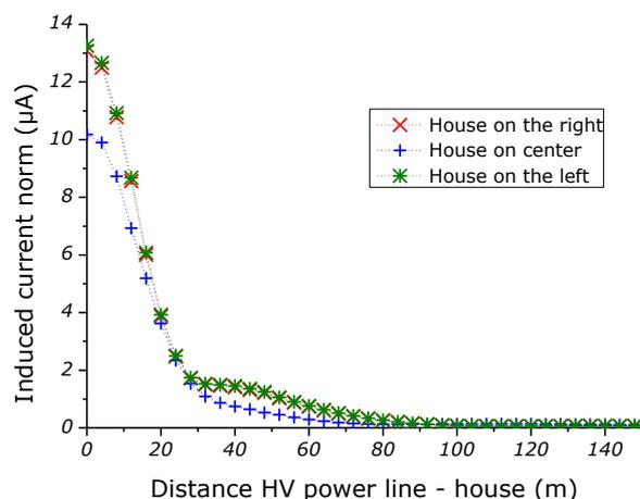
**Figure 17 : Induced current in the connections on the left of the house in the network on Figure 15.**
