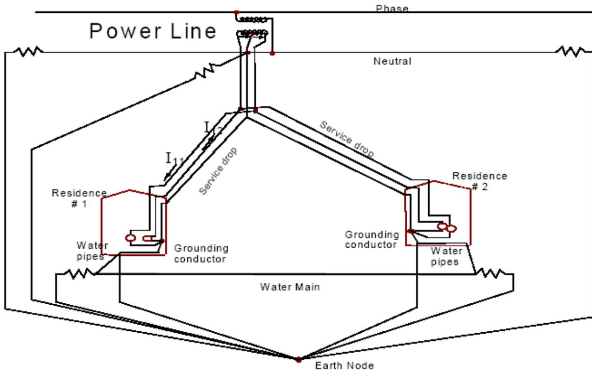
**Figure 21: Example of grounded network associated with the secondary wires.**
