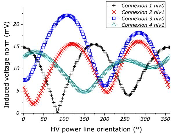
**Figure 8 : Induced voltage level in a single house as a function of the HV power line orientation.**
