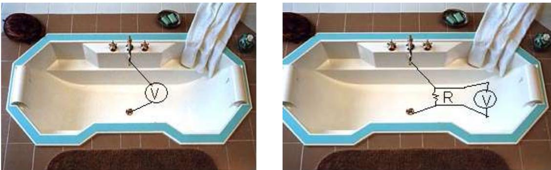
Figure 32 : a: Open circuit measurement b: Measure with 1 k $\Omega$  resistance
