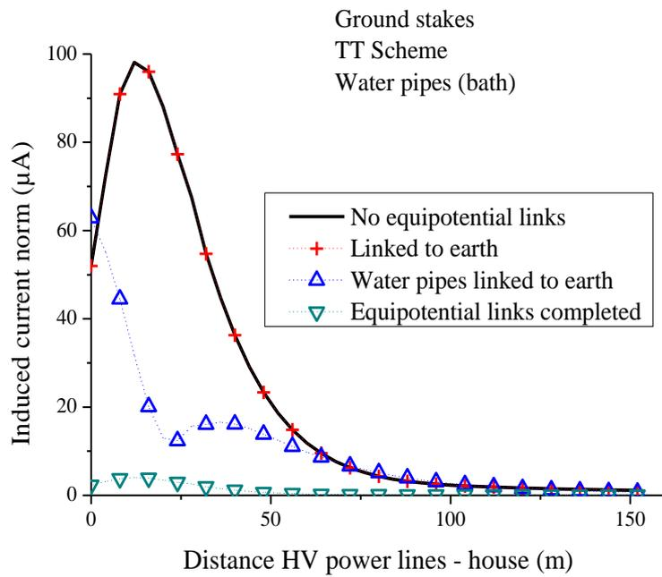
**Figure 30: Critical case of contact current level in a bathtub (Ground stakes).**
