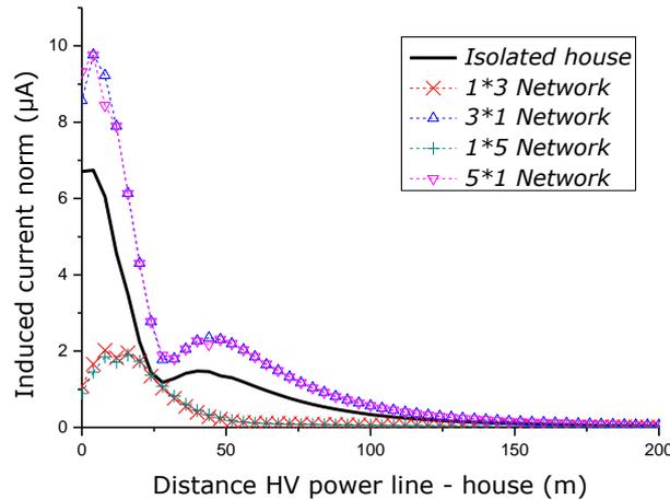
**Figure 12 : Induced current in connection 3 for different networks of houses.**
