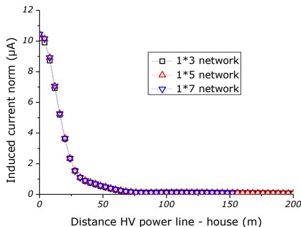
**Figure 13 : Comparison between induced currents in connection 1 in different networks of houses.**
