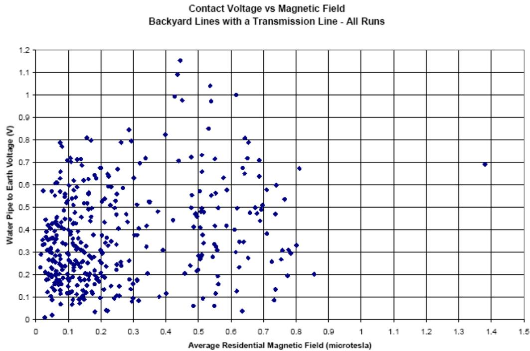
**Figure 23: Results with transmission line, low housing density and conductive water main.**
