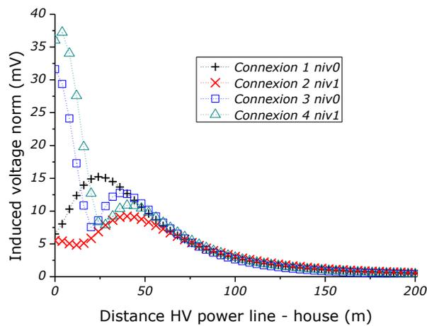
**Figure 7 : Induced voltage level in a single house as a function of the HV power line distance.**
