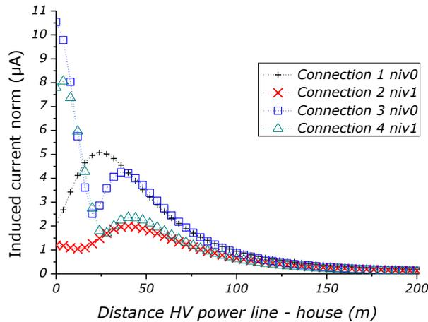
**Figure 4 : Induced current level in a single house as a function of the HV power line distance.**
