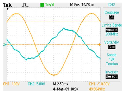
**b) Phase difference for a 100k resistor (cable length 5m)**
