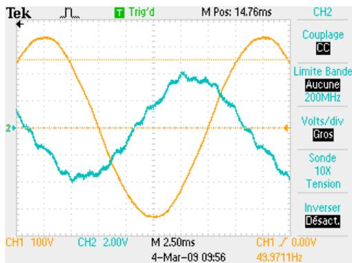
**Figure 43: a) Phase difference for 47k resistor(cable length 5m)**
