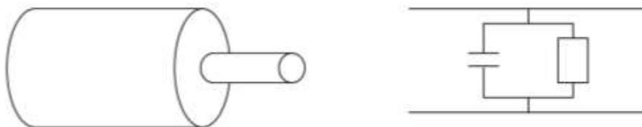
**Figure 41: Typical low voltage single phase wire and its model.**
