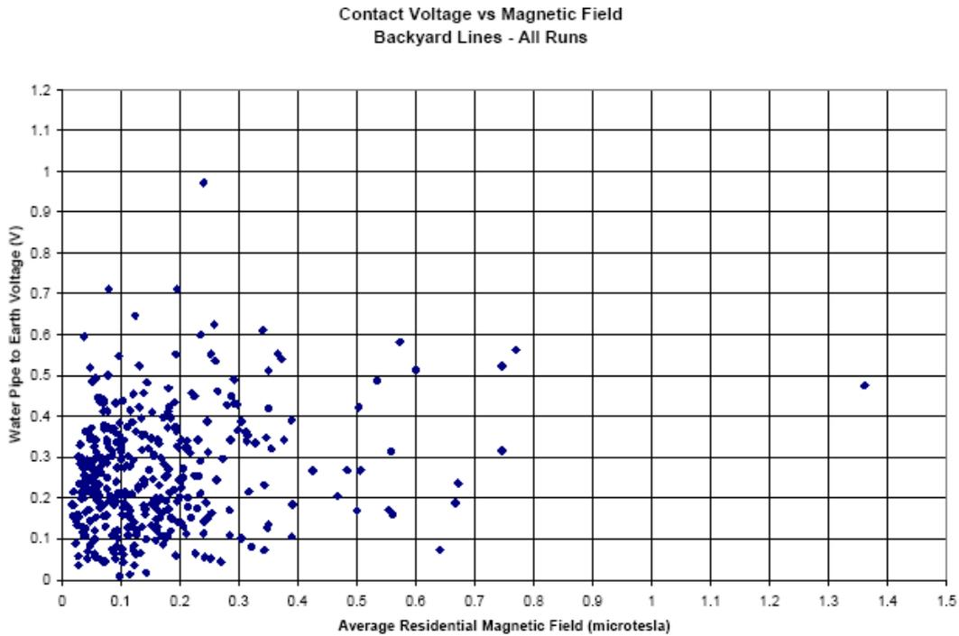
**Figure 22: Results with no transmission line, low housing density and conductive water main.**
