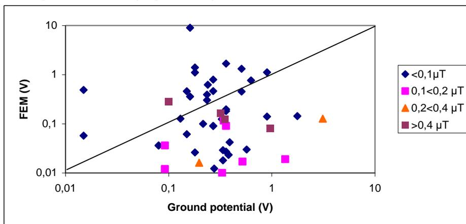
**Figure 40: Belgium campaign. The effect of ambient magnetic field on observed voltages**
