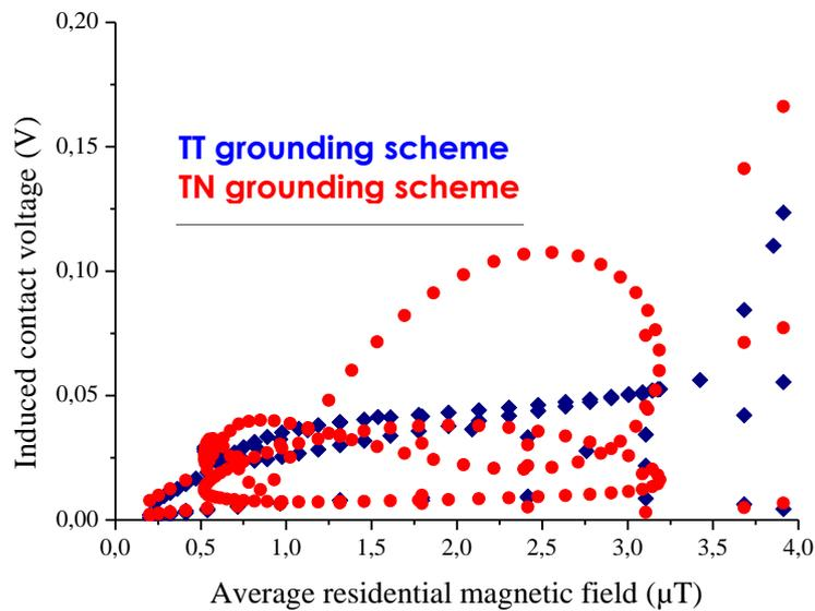
**Figure 27 : Contact voltage comparison on a wash machine in TN & TT grounding scheme in groups of houses with ground stakes.**
