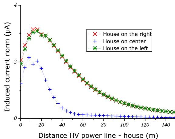
**Figure 16 : Induced current in the connections on the left of the houses in the network on Figure 14.**
