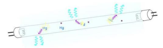
The UV radiation emitted by the mercury atoms electrons falling back in lower energy bands are absorbed by the fluorescent coating on the inside wall of the tube. The fluorescent material's electrons are in turn also excited: they jump from their unexcited state to a higher energy level (see <u>Electrical</u> <u>concepts</u>). When they return to their normal state, the released energy takes the form of visible light... we are enlightened!
