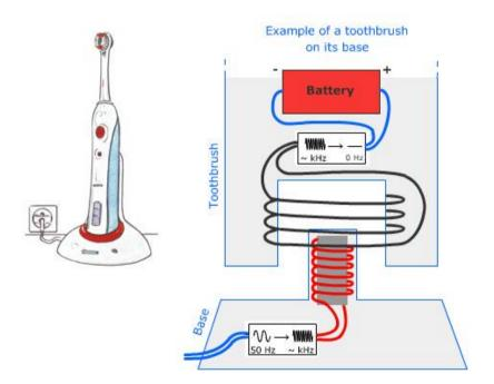
(See the Flash animation in <u>http://www.bbemg.be/en/main-emf/electricity-fields/uses-of-em-properties.html</u>) About 2 W of power is thus supplied to recharge the Ni-MH type battery.
