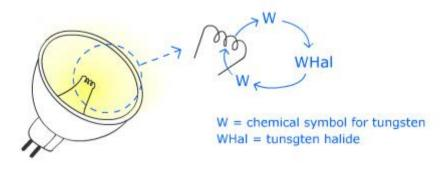
Thanks to this clever process, the filament can function at higher temperature (really higher, watch for burns!) while its useful life is increased.
