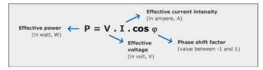
The phase shift factor, more commonly called the "power factor" is related to magnetic phenomena in motor windings.
