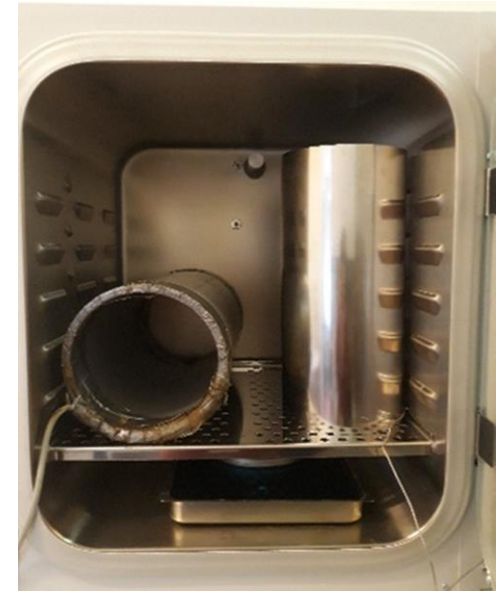
Picture of exposure system (left) and shielding system( right) inside incubator
